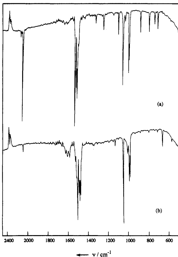
Figure 1. (a) IR spectrum of 1a matrix-isolated in Ar at 10 K. (b) IR spectrum obtained by irradiation of 1a in Ar at 10 K.
